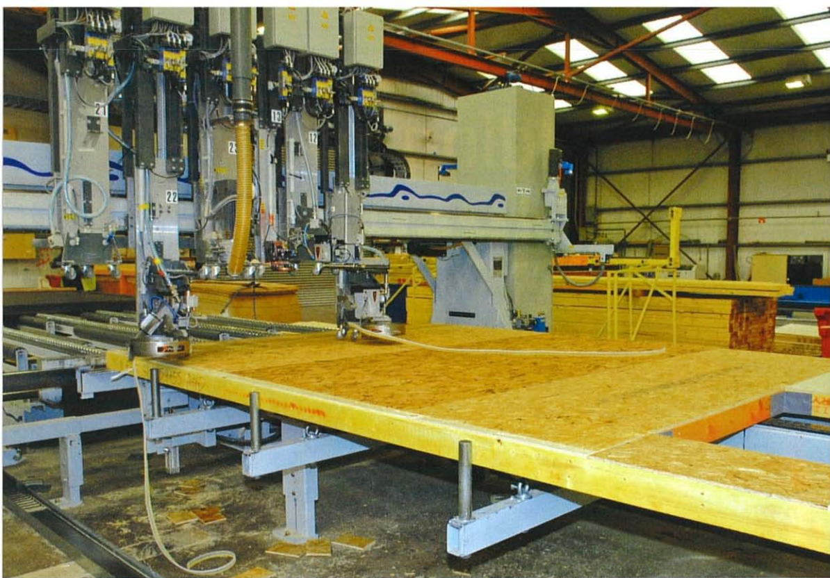
Factory assembly of timber frame panels
